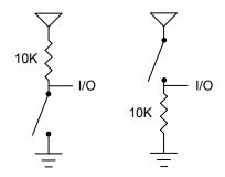
' Goto notpressed if button not pressed on Pin2 **BUTTON** PORTB.2,0,100,10,B2,0,notpressed
