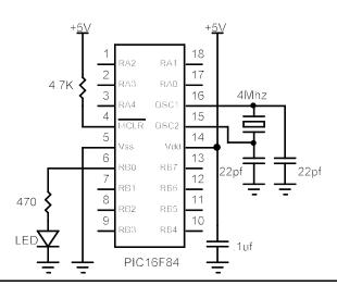
Build and double check this simple circuit on a protoboard and plug in the PIC MCU you just programmed. Our line of **PICPROTO**™ prototyping boards is perfect for this kind of thing.
